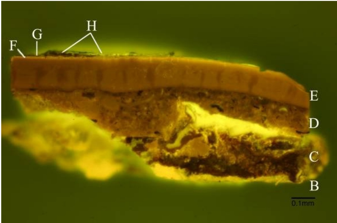
Figure 4 Cross-section of gilded area, 40x magnification, Blue light illumination
